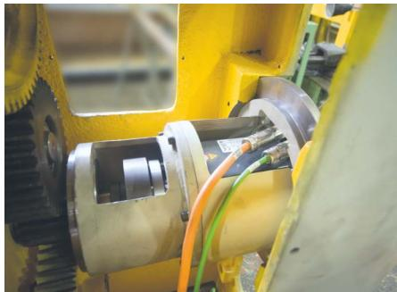
In the modern machines we are using advanced servo drive, which makes it considerably easier to adjust and increase the accuracy and operational speed. In addition, the usage of an electrical drive makes the machines easier to maintain and enhances its reliability.
