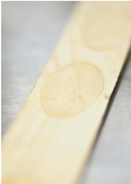
The machine is designed to improve the quality of the veneer sheet by cutting down knots and other defects of the sheet and replacing them with an insert from a specially selected veneer strip.
